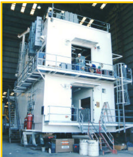
Offshore Production Module with 5KV & 480 VAC Switchgear
