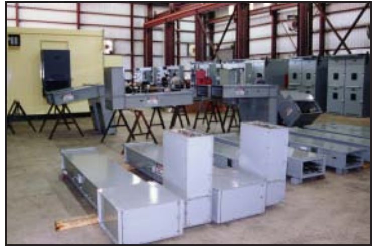
Low Voltage and Medium Voltage Bus Duct
