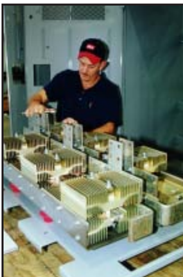
SCR Bridge Assembly
